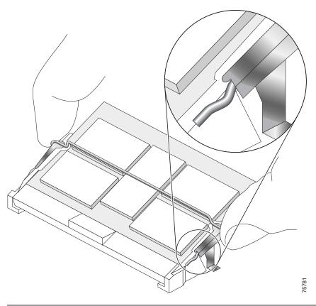
Figure 58 Retaining Clip Completely Installed into Module Latch
